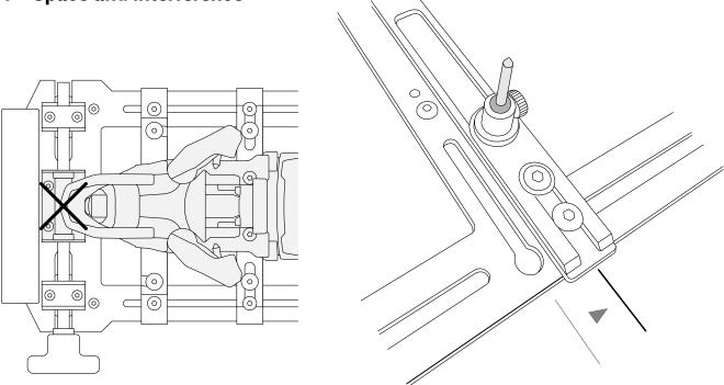
Particular ski bindings combined with large boots could cause interference between their pieces and the components of the jig's centering mechanism.
