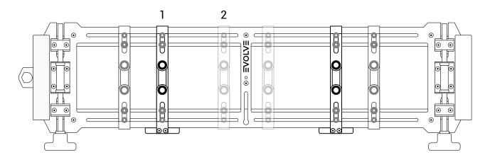
1) The two squared bars are in charge of maintaining the orthogonality of the binding. It's therefore necessary to always use these bars and keep them with two bushings installed.
