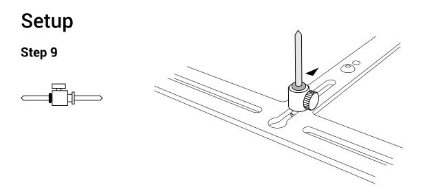
Insert the center indicator into its slot and bring it close to the ski boot. Set its height to get it as close as possible without it touching.
