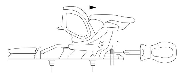
With piste or hybrid ski bindings, it's necessary to consider the heel piece's preload for an accurate hole positioning.
