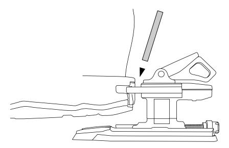
Most tech bindings require leaving a gap between the boot and heel piece. The manufacturer typically indicates the gap size in the binding specifications.
