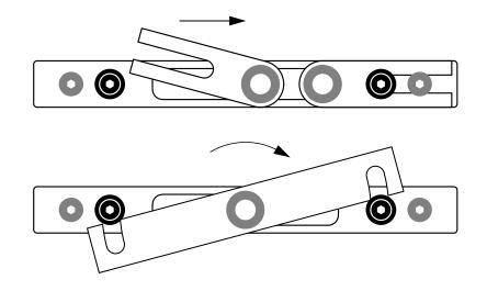
Where the binding hole pattern includes a centered hole, remove the bushing sliders and insert the central bushing holder.
