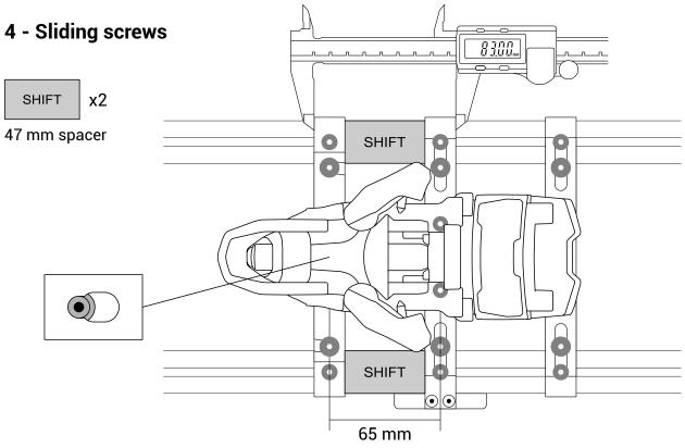
Some ski bindings feature mounting screw holes designed to accommodate the ski flex. When it is not possible to fix these holes in a neutral position, it is preferable to set their location on the jig through a specific procedure.
