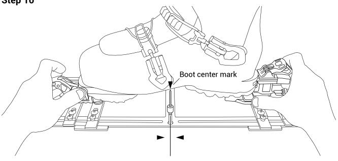
1) Slide the entire setup until the center of the boot is aligned with the indicator.
