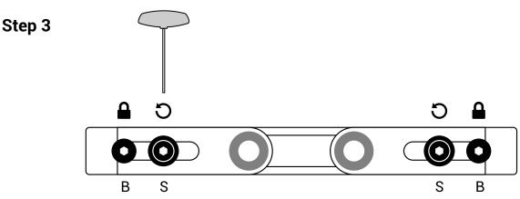
Unlock all the bushings sliders that will be used by loosing the internal screws on the bars (S).
